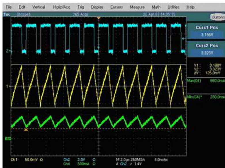
Figure 21. Electrolytic 100 \mu F (Ripple Too High)
