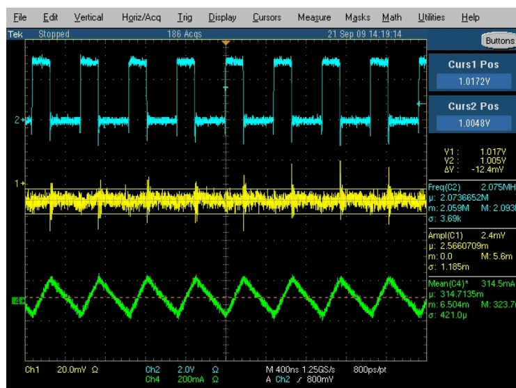
Figure 15. L=GLK2510P-2R2M, C=Ceramic 4.7µF 0805 X5R TDK (Ripple 12.4mV)
