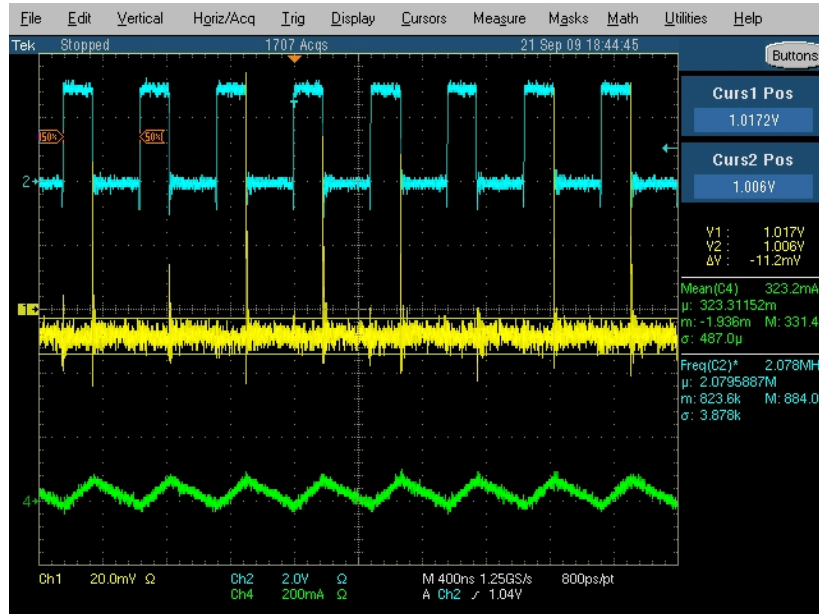
Figure 18. L=GLK2510P-4R7M, C=Ceramic 10 \mu F 0603 X5R YAGEO (Ripple 11.2mV)
